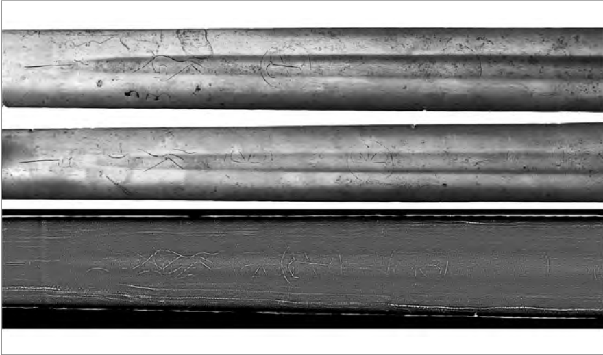
Fig. 4. Section of the blade with maker's marks and corresponding x-ray image revealing also welding lines. Photo by P. Žákovský.
