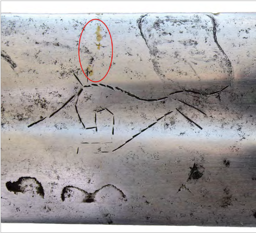
Fig. 7. Traces of brass that accidentally filled depressions not associated with any maker's mark. Photo by P. Žákovský.
