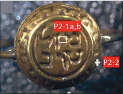
Fig. 8. Marked areas of EDS chemical analysis of the bottom of the ring with the inscription MAZAL TOV , photo and study by J. Michniewicz.
