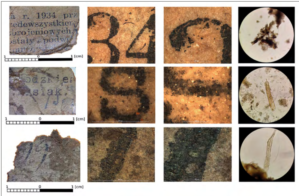
Fig. 4. Compilation of products on a paper base under the microscope (with reflected and transmitted light), visible mineralisation of samples (photograph by M. Majorek).
